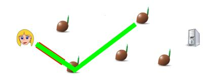
Alice tells n2 to contact a third node (n3), and establishes a new encrypted communication channel to n3, tunnelled within the previous one to n2
