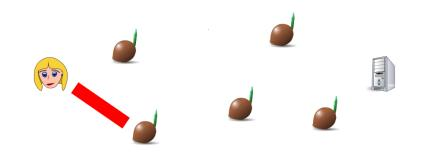
Alice tells n1 to contact a second node (n2), and establishes a new encrypted communication channel to n2, tunnelled within the previous one to n1
