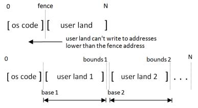
"user land n" can't write to addresses lower than the "base n" address or higher than the "bounds n" address
